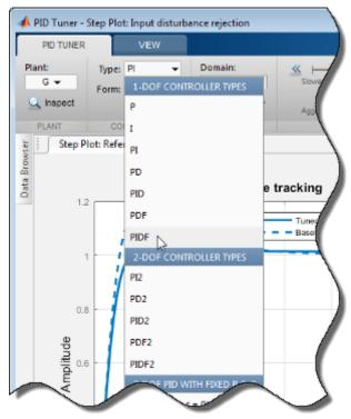
PID Tuner automatically designs a controller of the new type, PIDF. Move the **Transient Behavior** slider to set the coefficient back to 0.6.
